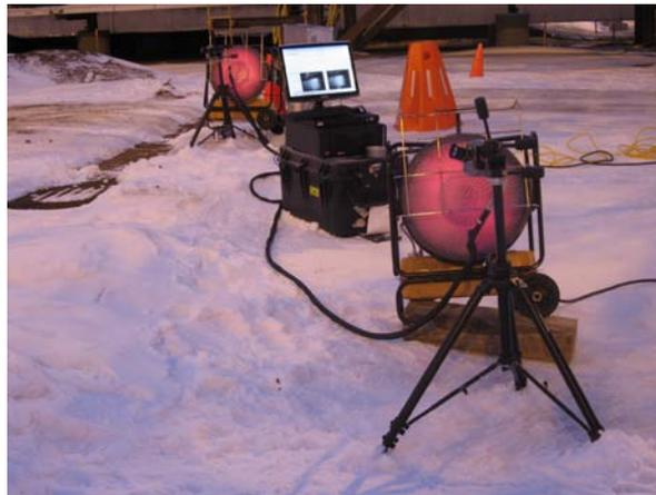
Figure 19: The stereo camera setup in the field, with kerosene heaters to enable camera operation far below their normal rated temperature. Temperature-controlled enclosures will be used in the future.
