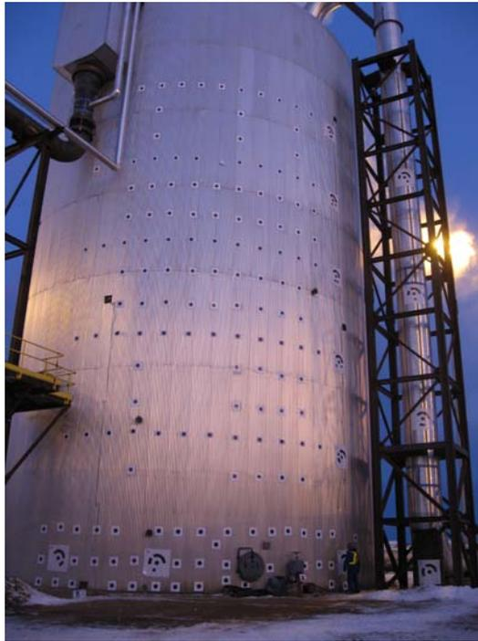
Figure 18: Six-inch dot targets and coded targets applied to 18 meter diameter x 23 meter tall water tank in order to determine the operating deflection shapes at various fill heights. Note the engineer at bottom right for scale.
